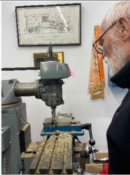
Craig Evans is machining journals which will go on the wheels he has made for the locomotive he is building.
