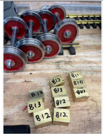
Craig Evans is machining journals which will go on the wheels he has made for the locomotive he is building.
