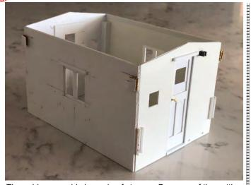
The cabin assembly is made of styrene. Because of the cutting required for doors and windows, the walls are laminates of thin sheets. The small black piece, upper right of the door is made of Plastruct square rod and drilled from above to create a snap-in holder for the ladder.
