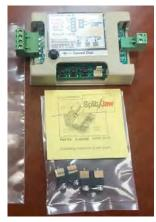
a stop. Track ends are sensed using a pair of Split Jaw insulating rail clamps, plus easy to install diodes (all included). An optional weather-resistant enclosure for the controller is available for outdoor use.
