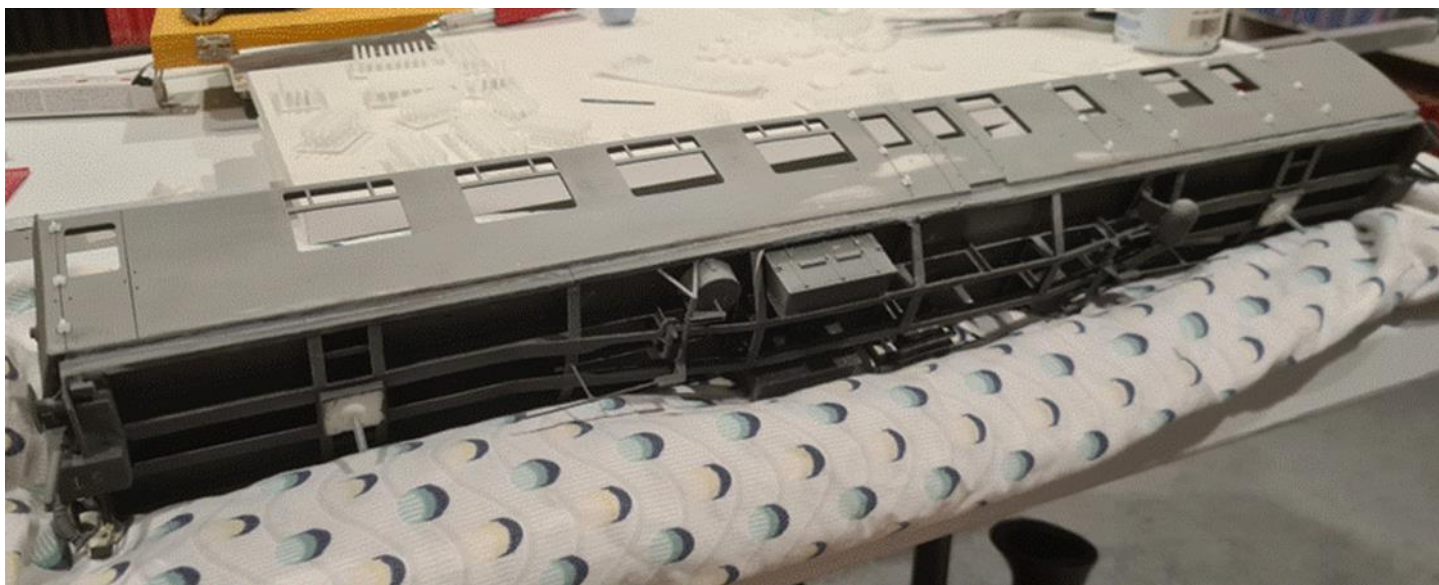
The brake corridor second with a primer coat and door hinges fitted ready for a final prime.
