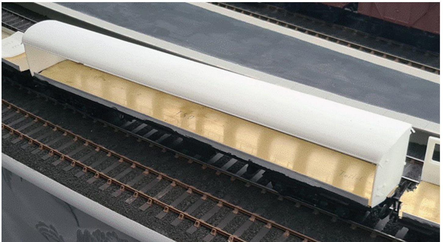
The assembly has now had the roof test mounted to check the fit. Note the toilet reference written on the floor on the right side. These are easily identifiable on the sides with their unique window arrangement.
