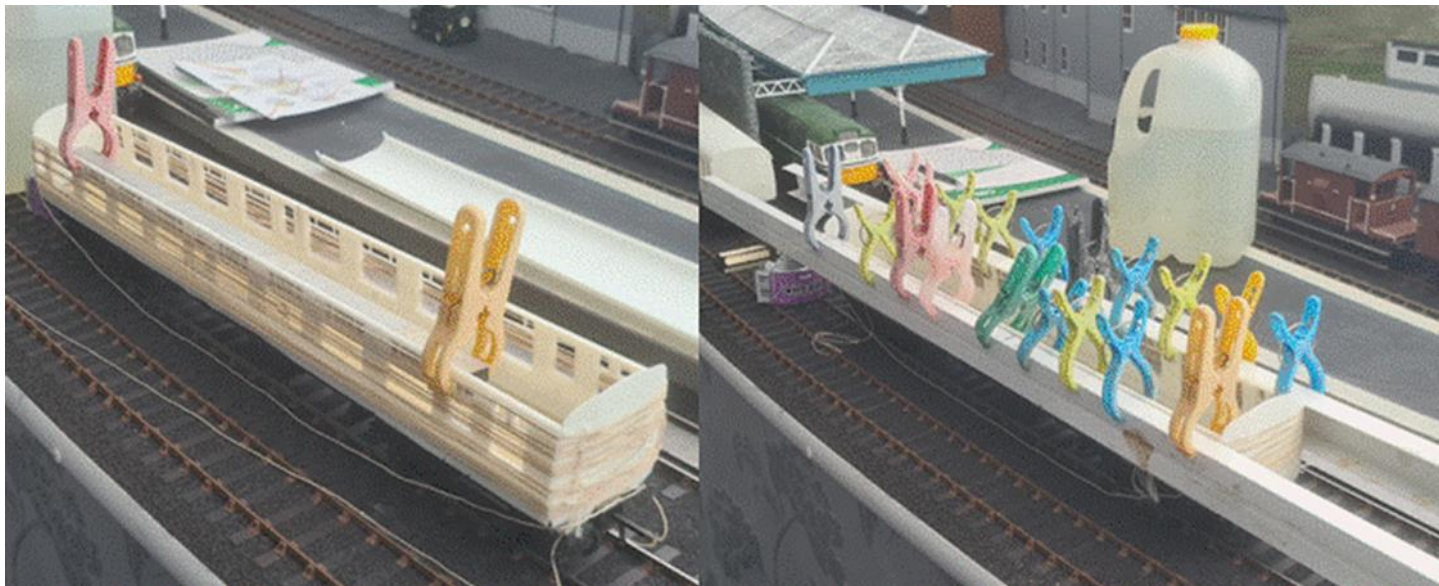
On the left, an early iteration of the straightening bracing. On the right, the adopted solution using channel sections to accommodate the curves of the sides as a real belt and braces approach.
