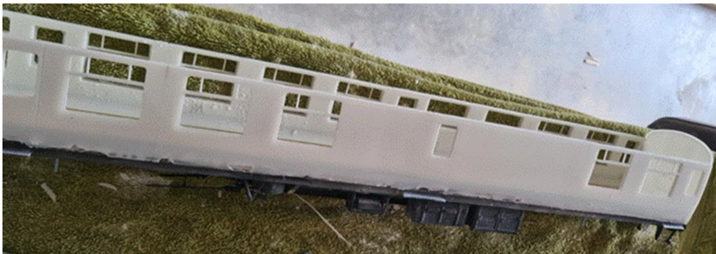
Bodyside sanded down roughly with footboards cut off.
