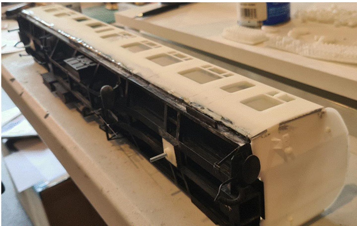
More araldite applied and left to harden for two days.
