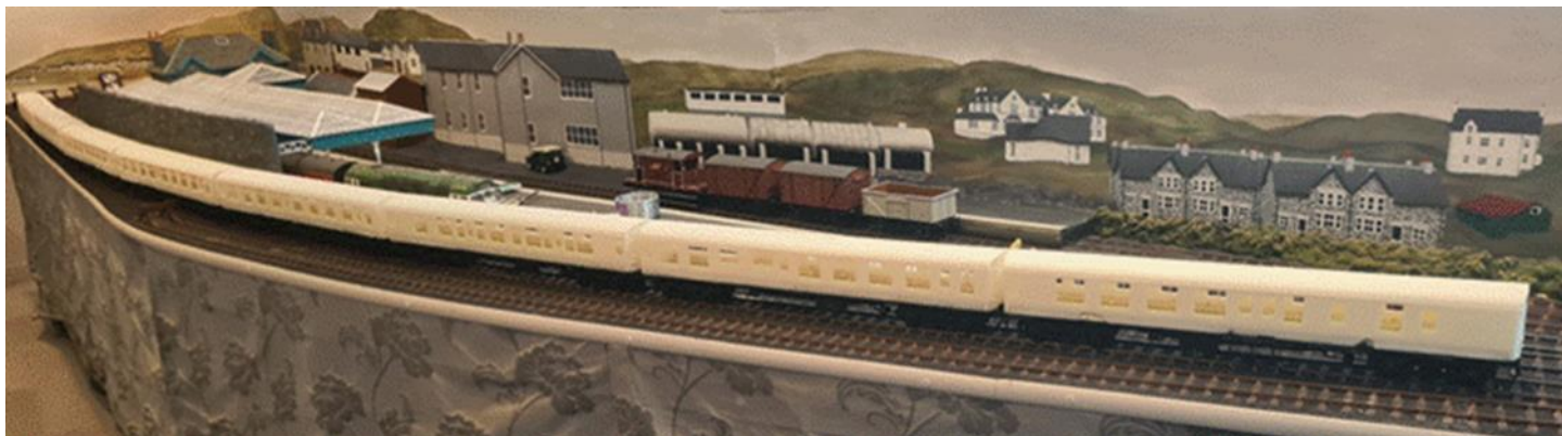
The full rake of eight carriages assembled and sanded smooth ready for priming. N.B. the roofs have been temporarily placed on top for the photograph.
