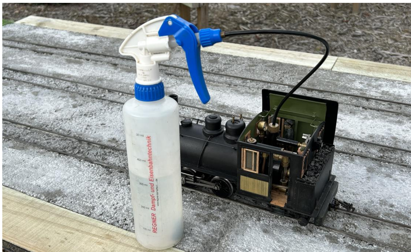
Regner bottle in use with my Accucraft Plantation loco Ngahere which uses a Goodall valve for topping up the water.
