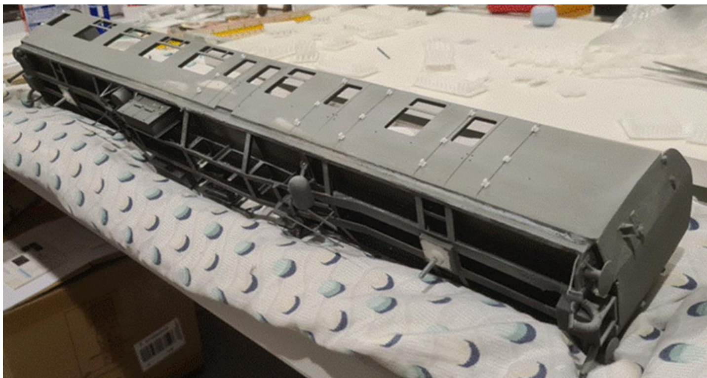
The BSK (Brake Second Corridor) fitted with hinges. Note the old sheet folded underneath to make a soft cushion for the hinges on the other side. Also note the instep under the guard's door in the centre of the carriage.
