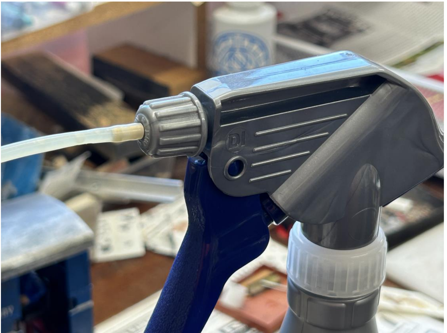
The barb fitted into the Spraymaster cap and hose fitted. (The correct hose this time!).
