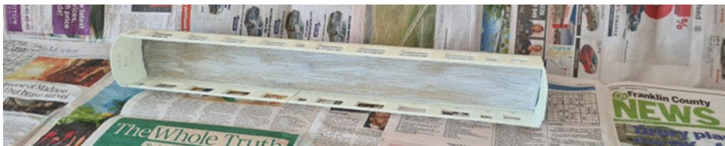
The white etch primer applied and the shell set up in a make do spray booth made up of old newspapers.
