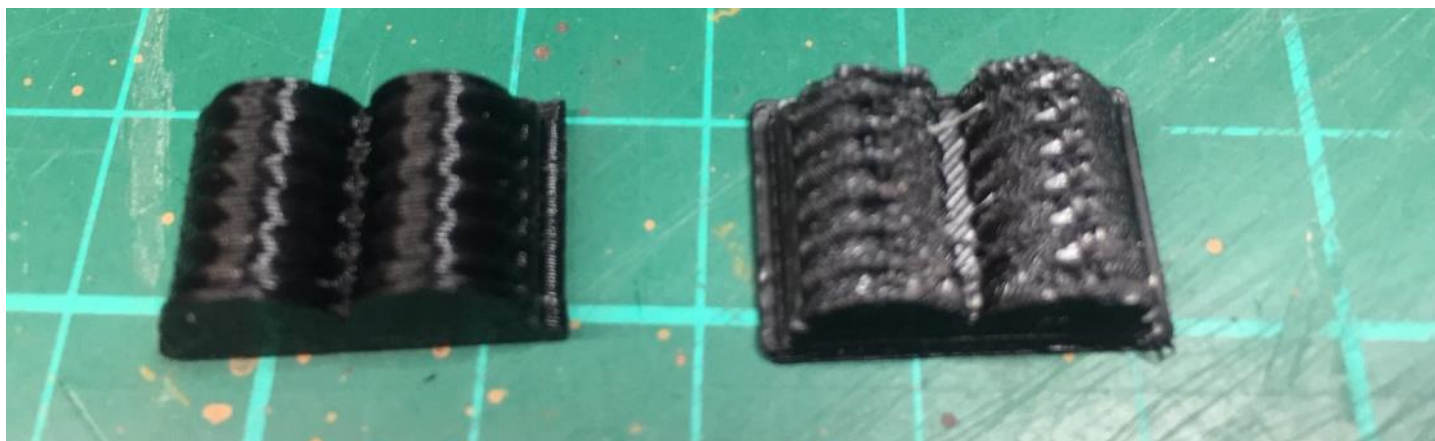
Left printed on end vertically, Right was printed flat as it is photographed.
