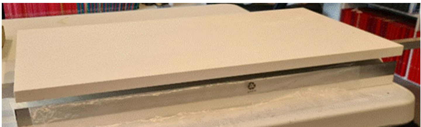
Shelving board in place to weigh down sections whilst glue sets and cures.
