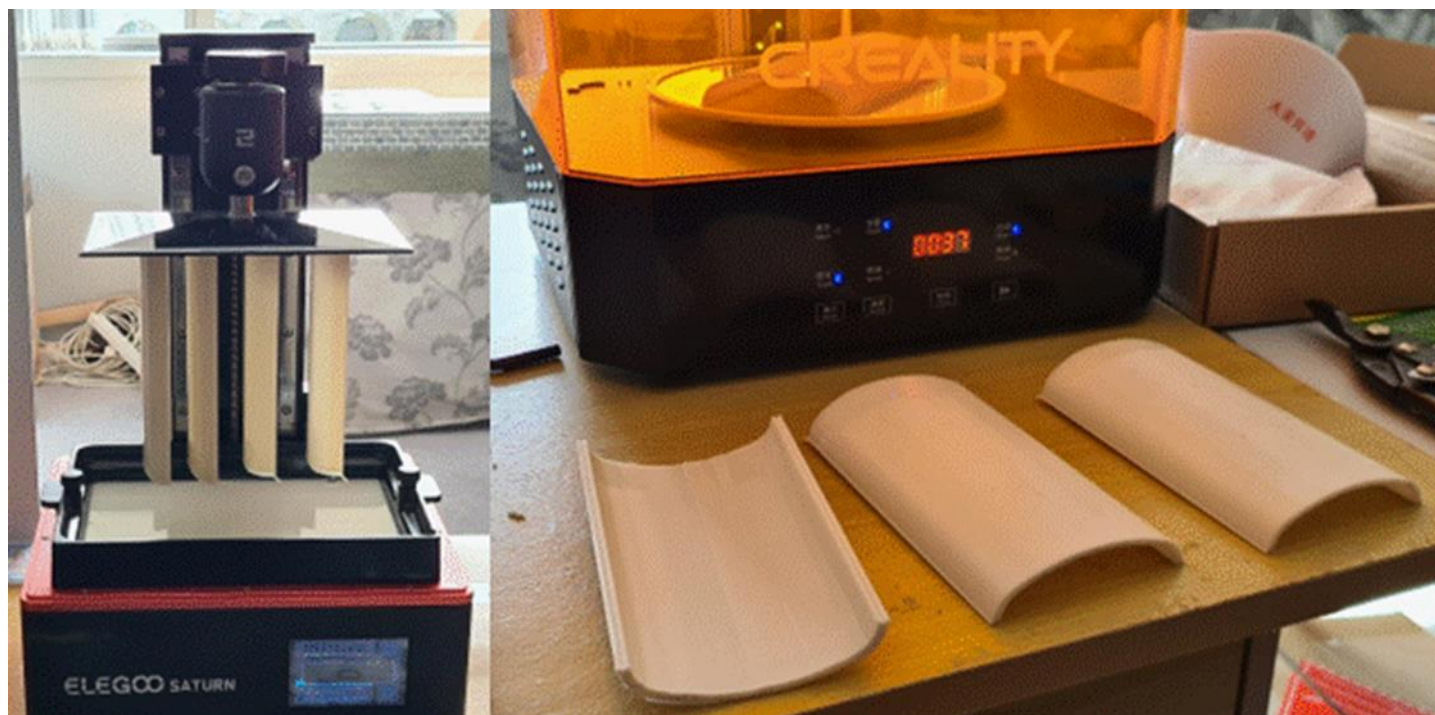
Printed sections for one carriage in the printer and, on the right, being cured. Note the height of each section has nearly maxxed out the printer!
