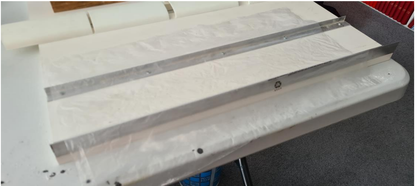
Roof assembly jig with polythene film placed over it.
