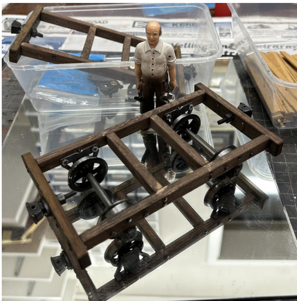
Left - Completed underframe to be used for a flat wagon following the Atropos style
