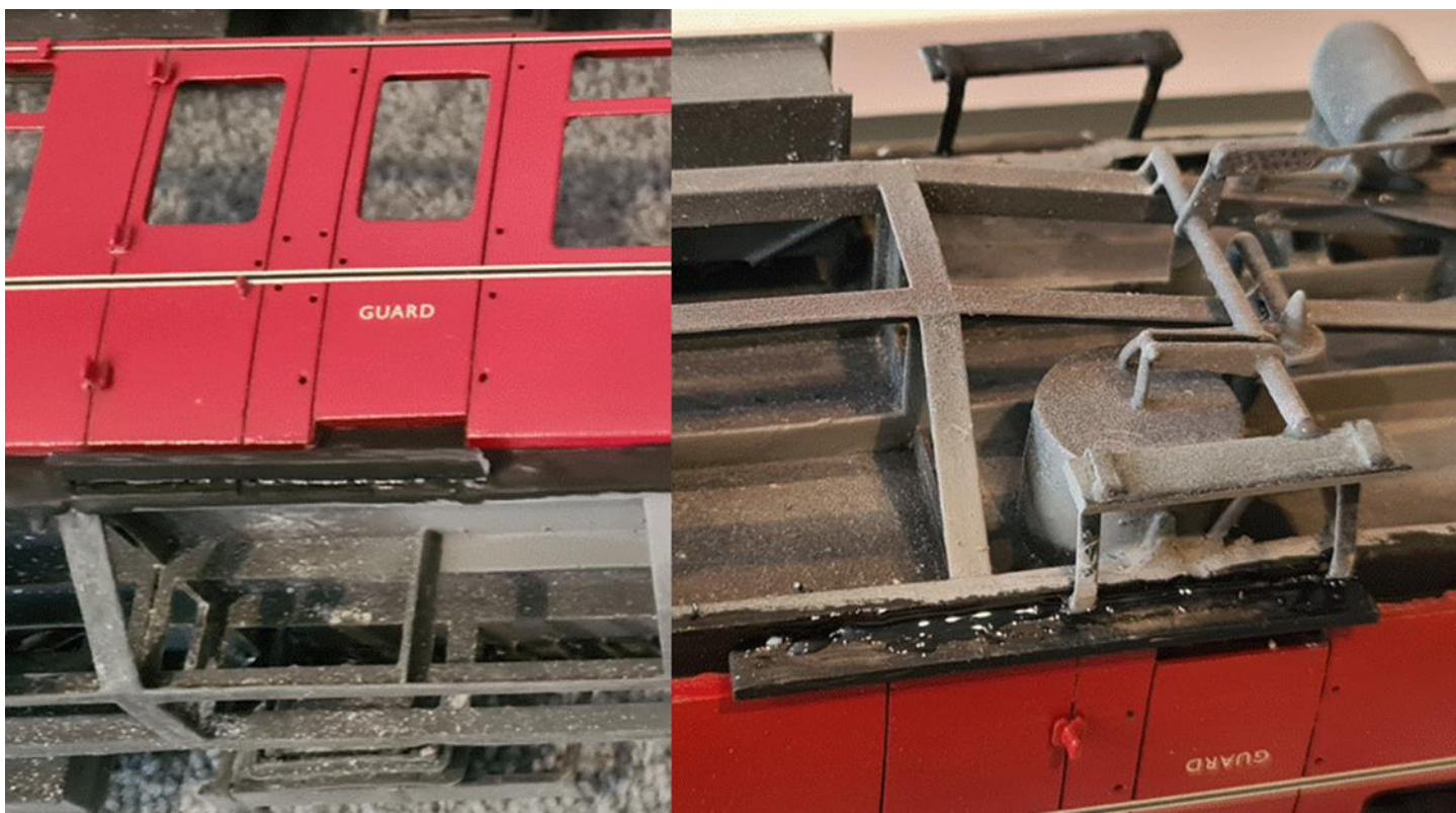
On the left, one of the missing guards' steps and on the right, reattached ready for painting again!
