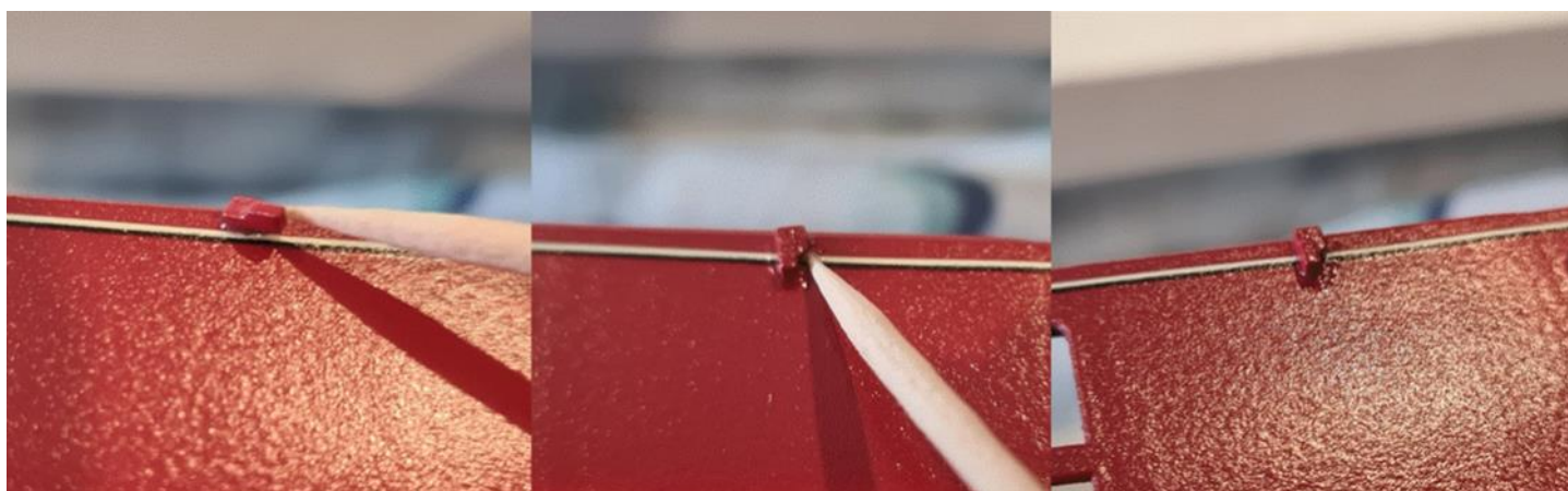
Moving the bracket into position, having smearing a drop of araldite underneath it. On the right, the installed bracket with the excess araldite removed.
