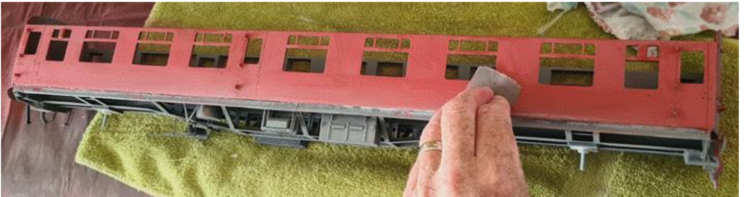
Rubbing down the first top coat prior to washing and applying a second.
