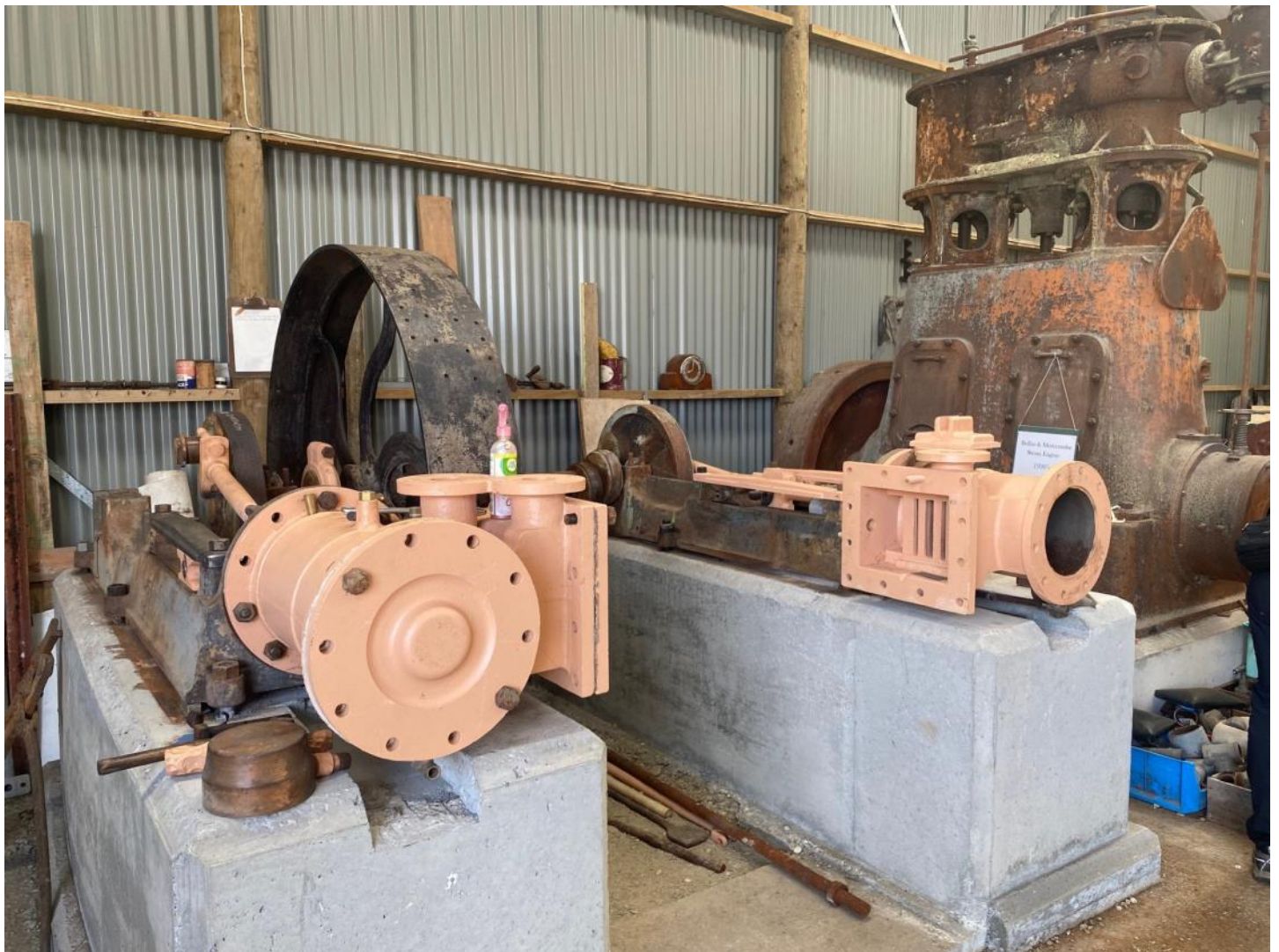
Twin Cylinder Engine that Jim is restoring at the Heritage Park - Photo Editor.
