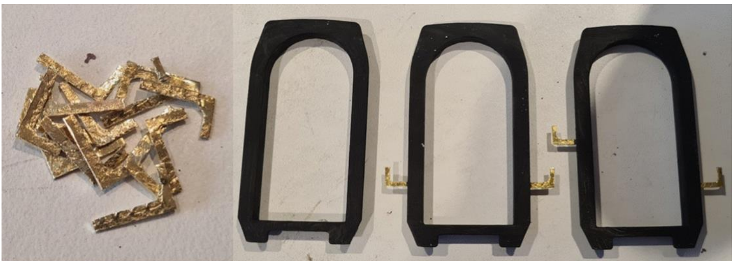
Batch of gangway mounted tail lamp brackets and the various mounting positions
