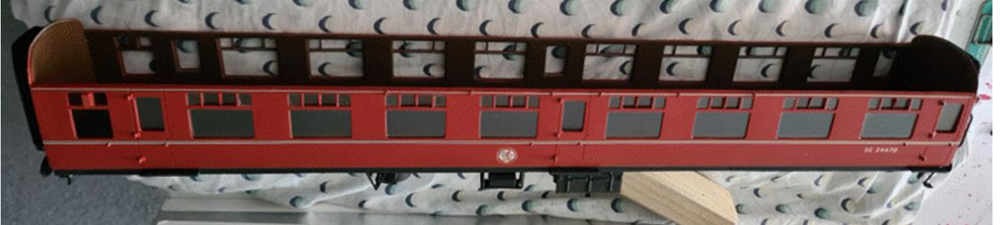
A SK second corridor with glazing fitted to one side.
