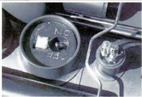
Figure 5: charging jack and power switch under the back steam dome
