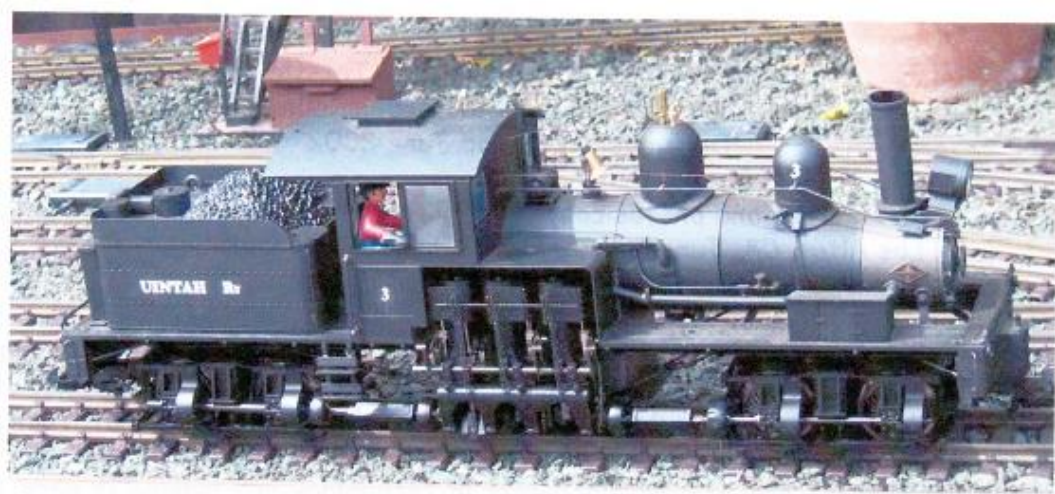
Figure 2: Bachman Shay with Uintah lettering. There are 12 sub-C nimh cells in the “tender” along with a Locolinc radio. The power switch is on the left front of the tender. The charging jack is under the coal along with the antenna. The auxiliary power input jack is at the rear of the water fill pipe. The weight was removed from the tender.
