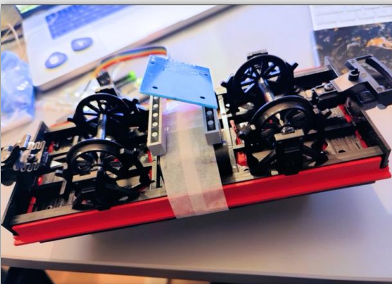
Measurement car with RC522 card reader, mounted approximately 3 mm (0.118 in.) from the track
