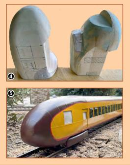
The front and rear of the train have complicated shapes, so I made those from basswood and finished with Bondo to make a smooth paintable surface (photos 4 & 5).
