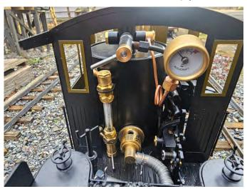
The pressure gauge and sight glass are easily readable. The sight glass has a blow-down valve.
