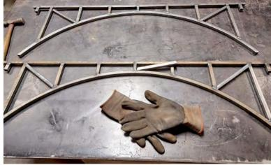
Photo 7 Fitting the cross braces.
