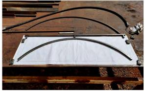
Photo 4 *Checking the beginnings of one side against the drawing of the gap to be spanned.*
