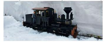
found on logging and mining railroads. They were also geared to run at much slower speeds than a typical rod engine, making them much better pullers. The Shay came in many configurations, from the smaller 10-ton 2-truck Shay to a 162-ton 3-truck Shay which still runs on the Cass Scenic Railroad in West Virginia.
