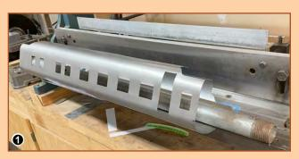
I drew up each car in a CAD file as a one-piece steel sheet metal part that had the windows and other profiles laser cut. The sheet was then rolled and bent over a steel pipe (photo 1) to form a complete tubular shell (photo 2).
