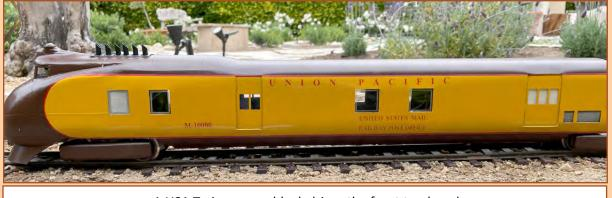
A USA Trains power block drives the front truck and 14.4V Li-ion batteries give well over an hour of running time.
