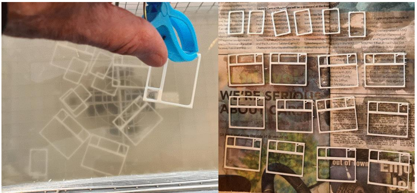
Left photo: a batch being cleaned in IPA. The clothes peg was particularly helpful in getting these in and out. Right photo: Batch of washed frames drying out.
