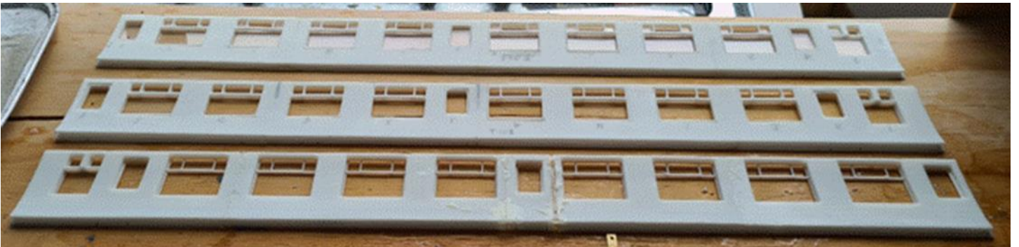
Stages of bodyside window frame fitting. Bottom: raw glued print. Centre: sanded bodyside with frames fitted. Top: glazing inserted.
