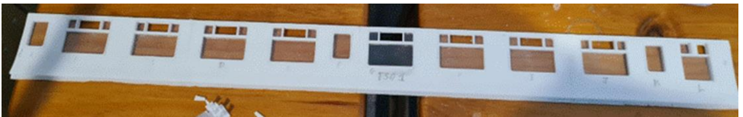
A bodyside with frames and glazing fitted with coach type and number and window numbers written on frame
