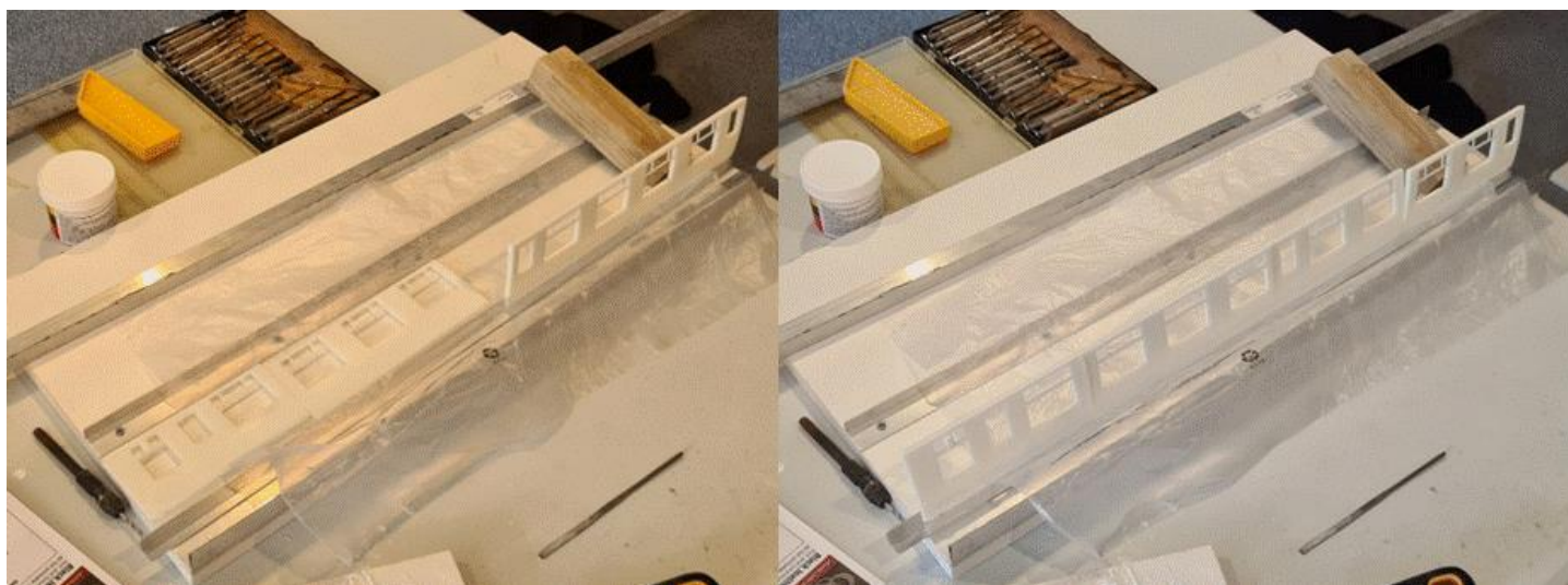
Assembly of panels with two fitted on the left and all four with glue applied and fitted on the right. N.B. the wooden block on the right of each picture is holding the assembly upright.
