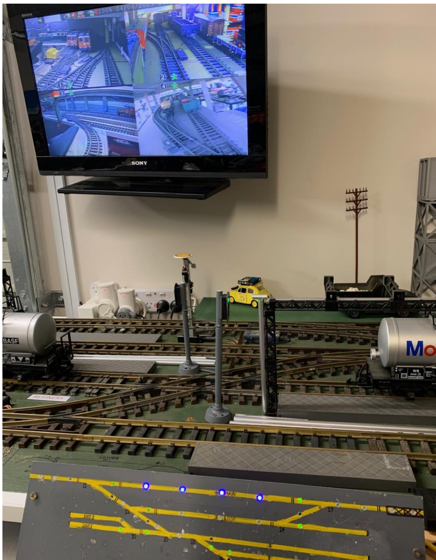
Controls for the lower level, note the screen with cameras to see if mainline is clear
