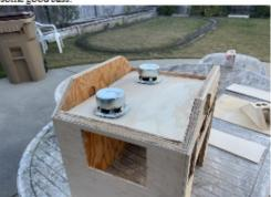
The speakers have an extended lip around the cone so when I cut the holes in the board, the speakers settle nicely into the holes. This gives them more stability beyond just screwing them down.
