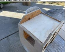
Here are the pieces to the framework for the roof. I custom cut the four strips from a scrap piece of pine. The notch in the front piece of plywood is to allow clearance for the bolts that attach the brow and for the wires from the lights. Pretty simple design.
