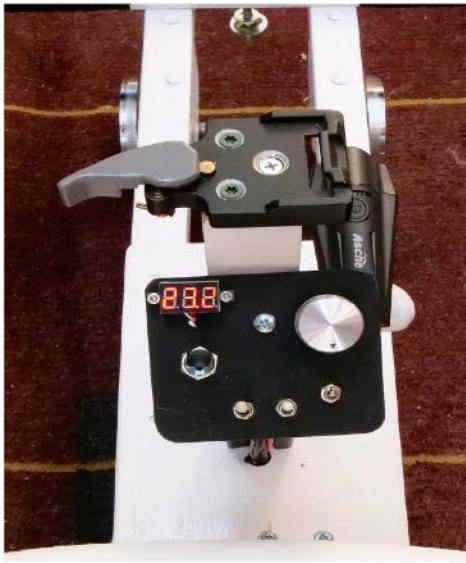
The control panel (speed, reverse, brake, etc.).
