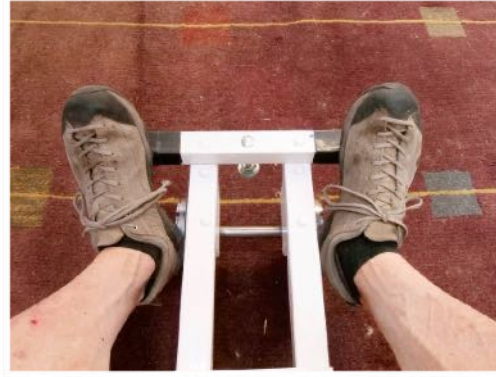
Foot brake in 'stop' position (Note: Heels are on the wheels)
