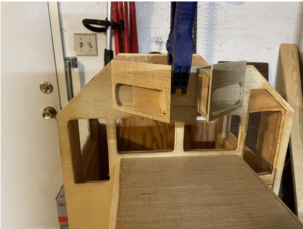
I made a notch at the back end of the supports for them to slide onto and around the hanger.
