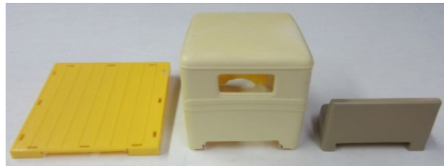
parts after cutting, grinding and fitting
