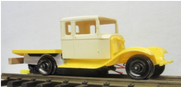
Preliminary run to check alignment & clearance
