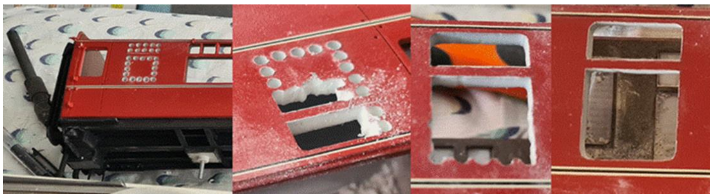
Montage of window carving to create the missing window openings. The holes were opened out from top to bottom to minimise excessive pressure on the thin top and dividing bar sections.
