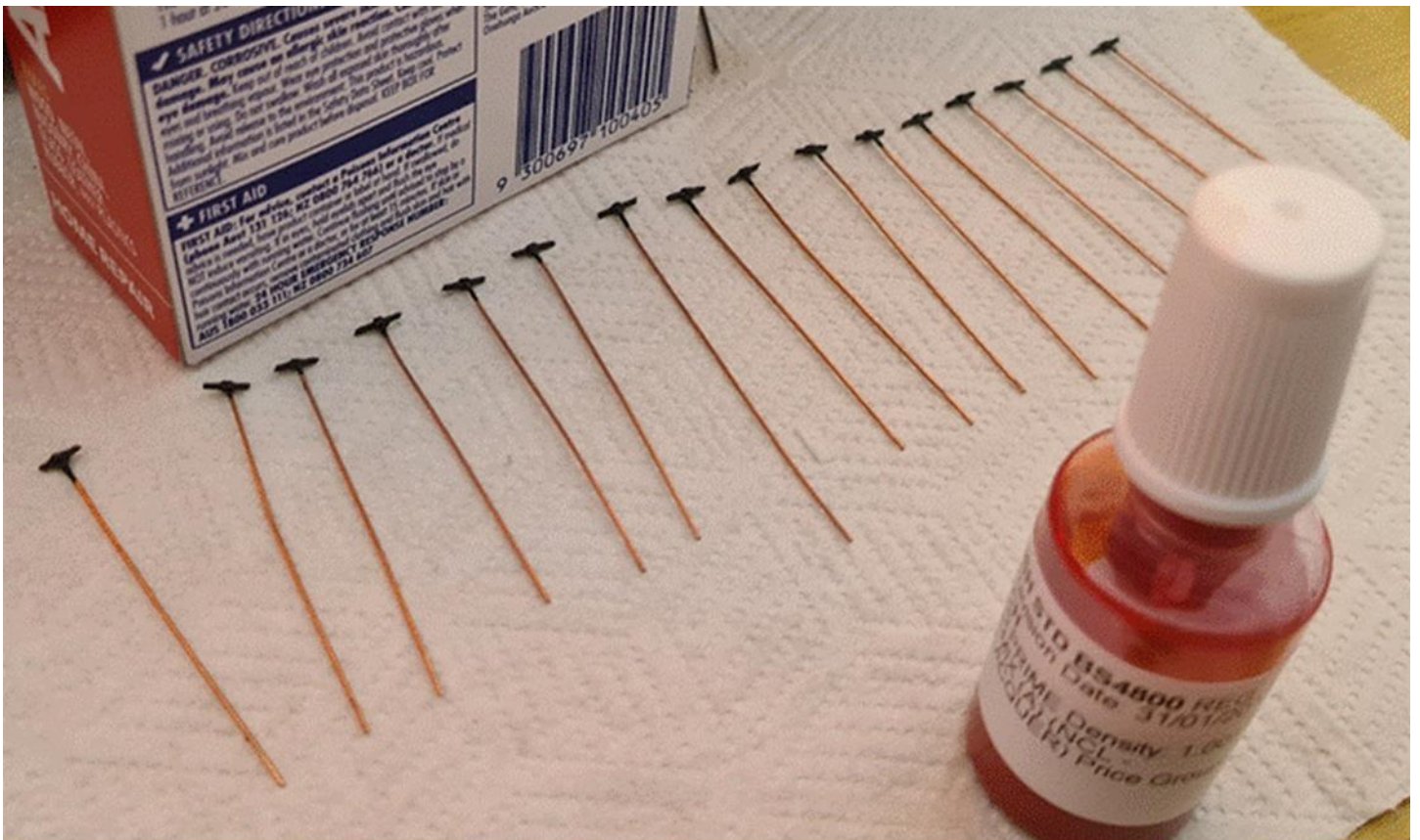
“Tell-tales” prepared and primed at the ends ready for the top coat.
