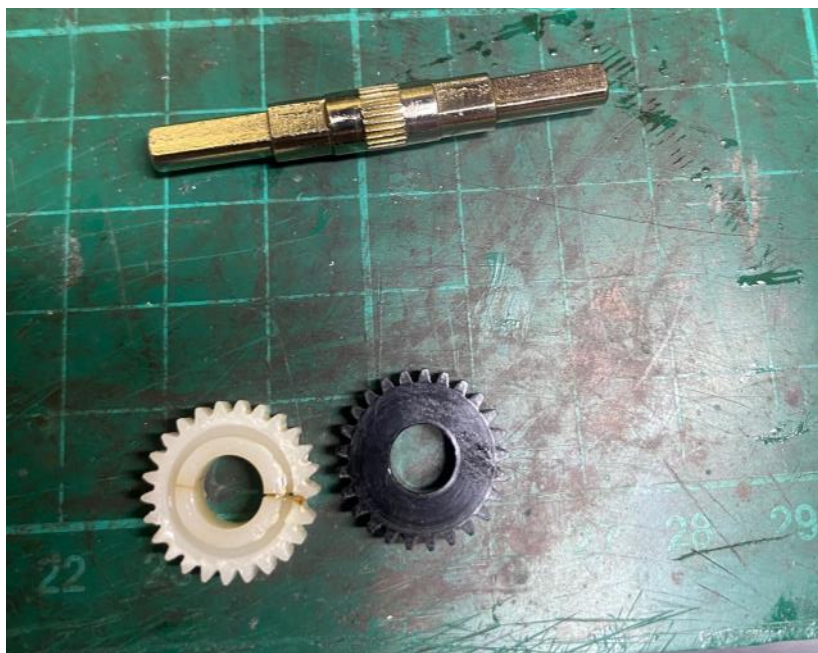
Left - split main gear on shaft from the gearbox. Right - Split Bachmann gear versus the replacement gear from Northwest Short Line.
