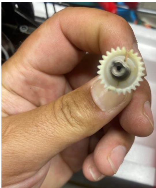
Left - split main gear on shaft from the gearbox. Right - Split Bachmann gear versus the replacement gear from Northwest Short Line.
