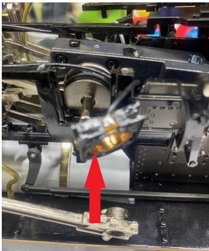
Left - Removing the pickup housing these just lift out of the frame, Right - Slide the concentric mechanism off the main driveshaft. Note the use of wire to hold parts together in correct order.
