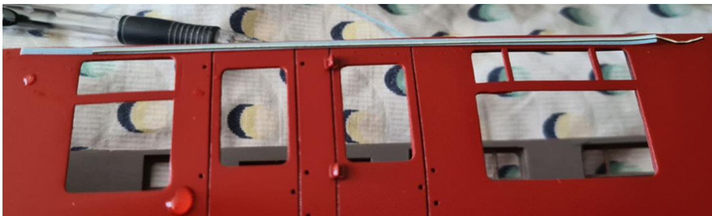
Decal with backing paper placed on the body in the roughly correct location. One end has been drawn off onto the body
