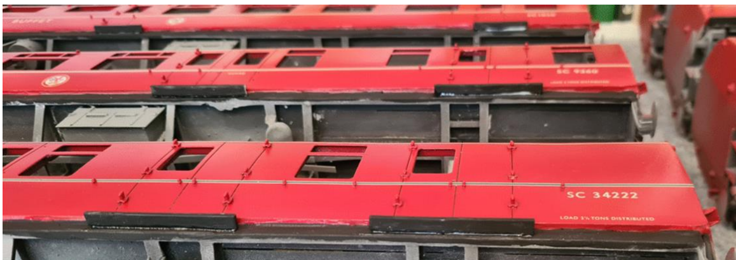
The BSK brake second corridor with door bumps and footboards fitted.
