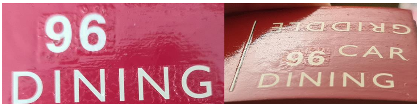
Trial decal application with the "96" on the left treated with a brush on varnish with disastrous consequences. The GRIDDLE logo on the right was the second attempt, this time using the same spray varnish used as the base. This showed some wrinkling after about the second to third spray. The third attempt with the DINING logo showed the same wrinkling on the left however with the technique described above I managed to remove all the wrinkles as can be seen on the right. The CAR logo was the fourth attempt and proved successful as well.
