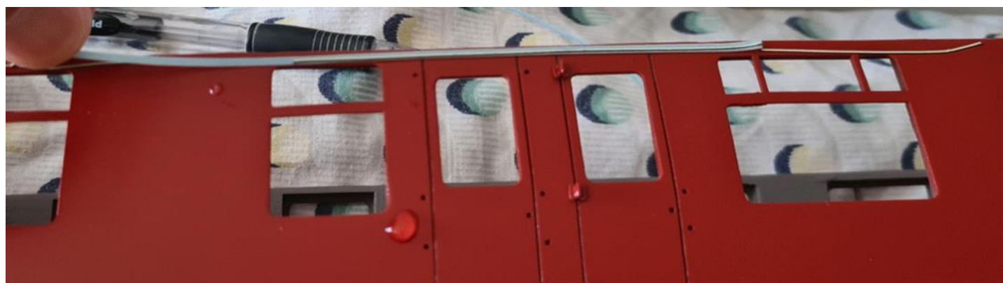
Sliding the backing paper off from under the decal leaving it in approximately the correct position
